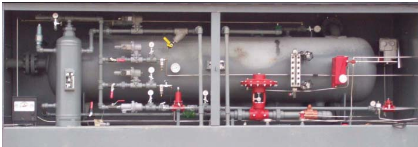
CNX Gas installed surface equipment Dec. 12, 2008, at the CNX No. 3, the company's first horizontal well, enabling it to flow at 6.5 MMcfd (Fig. 6; photo by Sam McLaughlin, CNX Gas Corp. vice-president, northern Appalachia operations).
