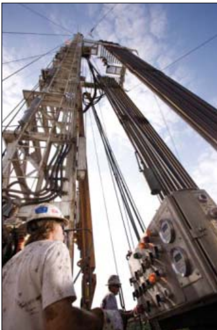
A driller operates a control panel board on Les Wilson Rig 25, drilling a Marcellus shale well in Pennsylvania (Fig. 3; photo by Harry Giglio from CNX Gas Corp.).
